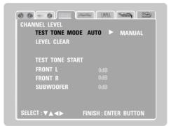
Use the ◀ and ► cursor buttons to select "Auto" or "Manual" for the "Test Tone" mode. • The selected setting is displayed
